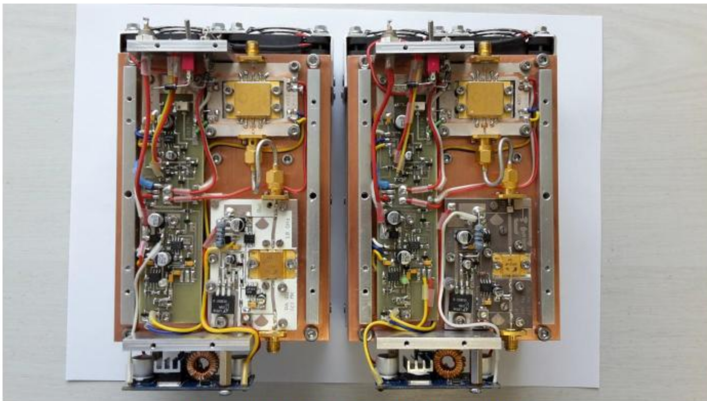
Figure 1. Two 10 GHz power amplifiers with TGA2312FL
