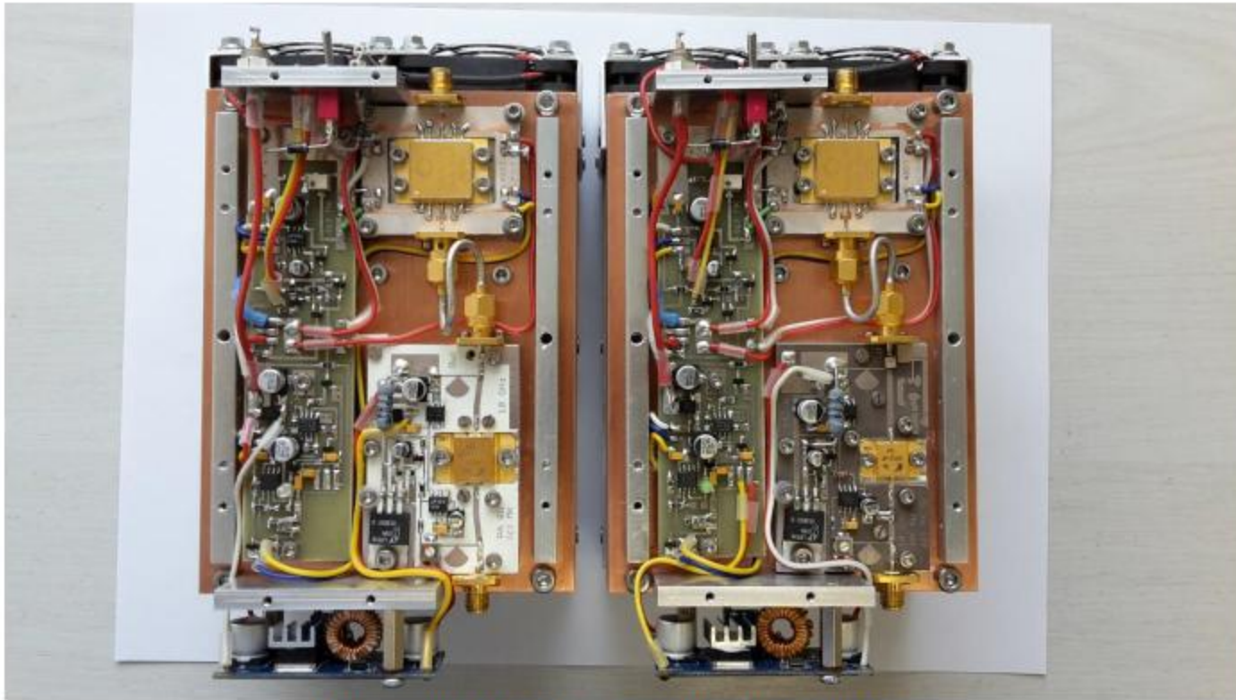
Figure 1. Two 10 GHz power amplifiers with TGA2312FL
