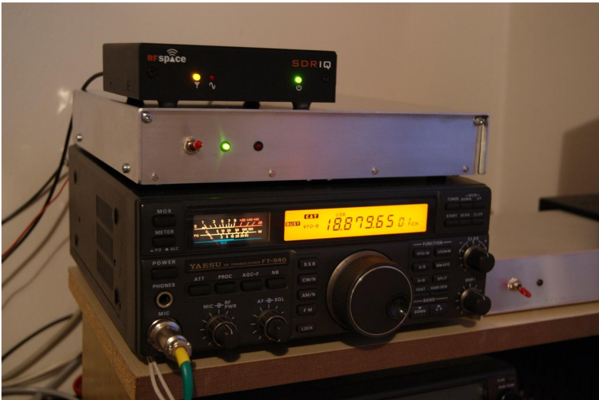
Figure 5. EME receiver SDR, transverter and IF transceiver
