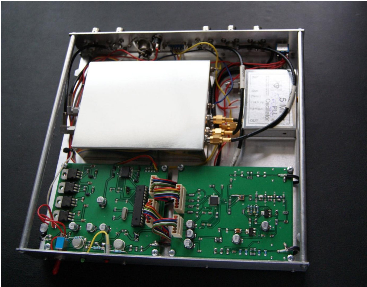
Figure 4. 144-149 MHz/14-19 MHz Transverter
