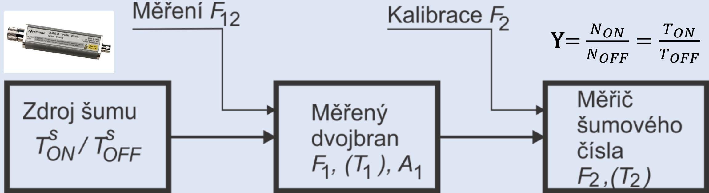
$$ENR = \frac{T_{ON}^s - T_{OFF}^s}{T_0} \quad [K]$$
