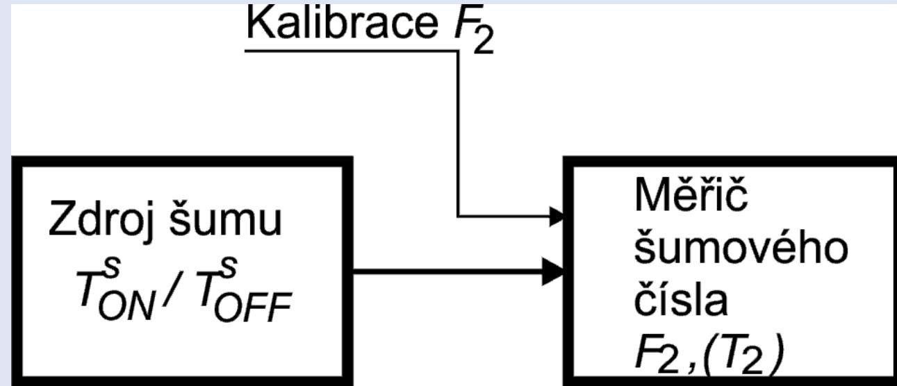
$$Y = \frac{T_{2ON}}{T_{2OFF}} = \frac{T_{ON}^S + T_2}{T_{OFF}^S + T_2}$$
