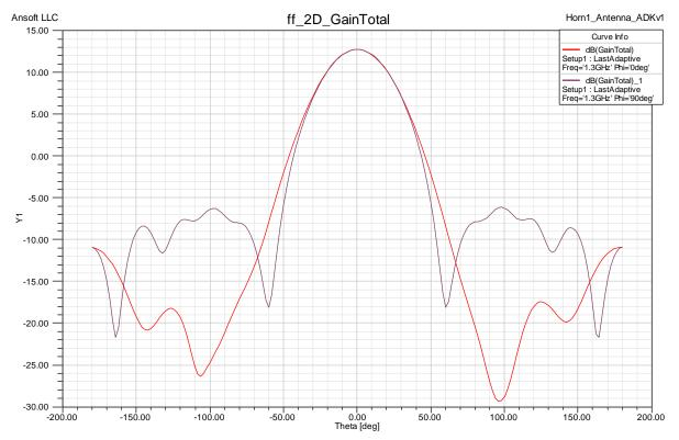
Fig. 1. Radiation pattern of the extended septum feed by horn.
