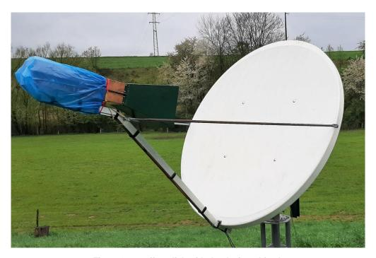
Fig. 3. 1,8 m offset dish with the designed feed.
