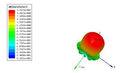
Fig. 2. 3D radiation pattern of the extended septum feed by horn.
