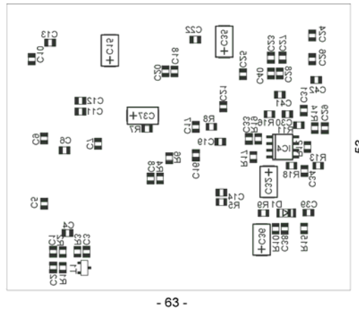
Fig. 8: Bottom layer of components
