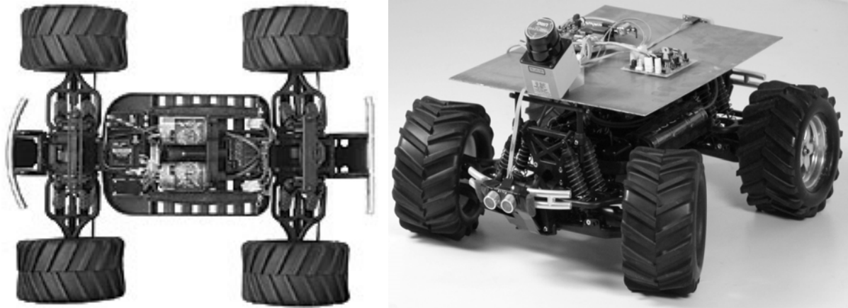
Fig. 2.2: Left - the original RC monster truck [4]; right - the complete robot with batteries, sensors and electronics.
