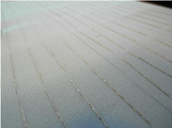
Fig. 4: Heating layer created by silver conductive thread.
