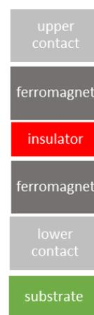
Fig. 1. TMR sensor structure.
