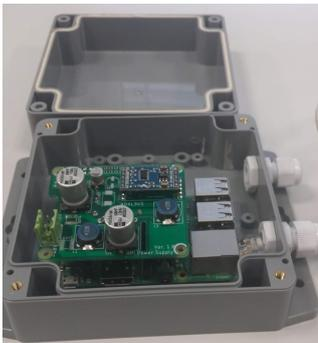
Fig. 2: Prototype of device for vibration measurement
