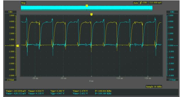
Fig. 9. Measurement of LM319 comparator outputs.
