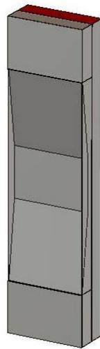
As can be seen, the only difference between the pressure and smoke detector are slots in the top metallic layer and that the textile in between top and middle metallic layer is taken away to provide purely air-filled cavity. This way the sensitivity of the smoke detector is better as smoke would hardly propagate through the textile layer.
