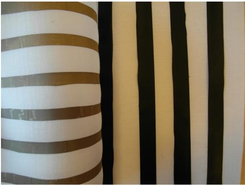
Fig. 2: Pressure matrix sensor based on piezoresistive foil; matrix 8x8.
