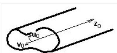
Fig. 3.1B.2 Longitudinally homogenous waveguide. u, v : transversal directions, z : longitudinal direction.
