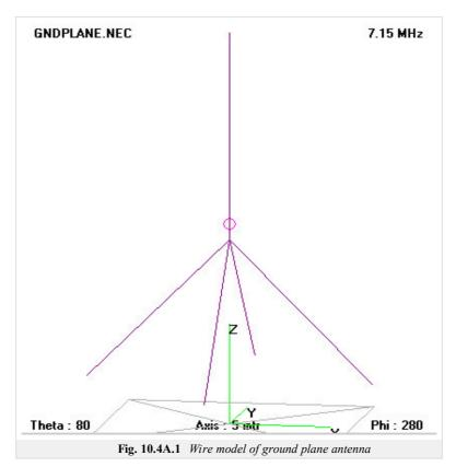
Far from the antenna and near the ground, electromagnetic fields and radiation patterns are the same as for a half-wave dipole. The impedance is not the same a with a good conductor ground plane. Conductivity of earth surface can be improved with an expensive copper wire mesh.
