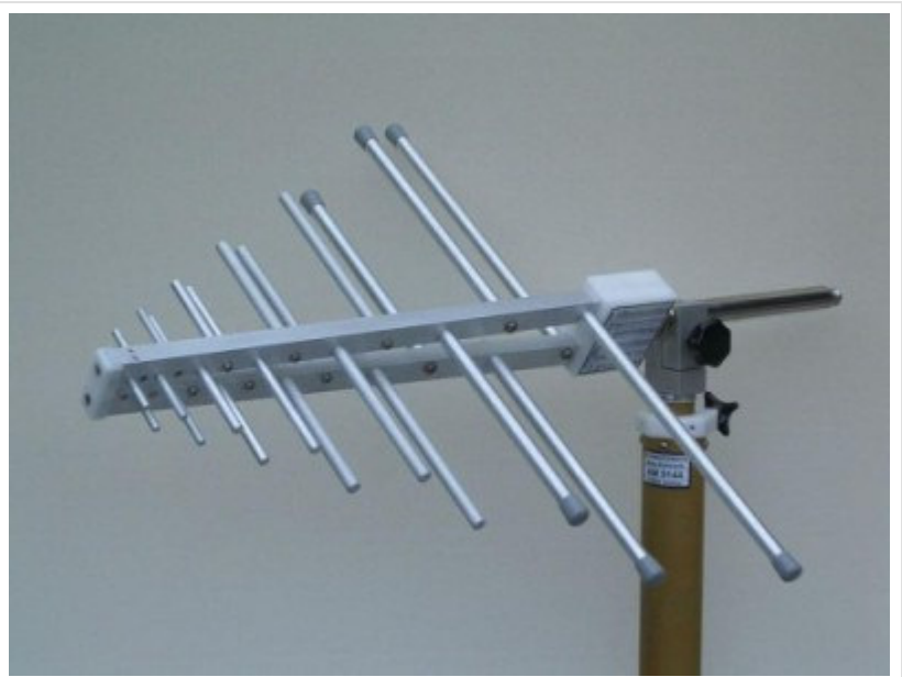
Fig. 10.8A.1 Practical implementation of LPA antenna
