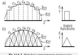
Fig. 4.1A.3 Multi-basis approximations a) piece-wise constant, b) piece-wise linear
