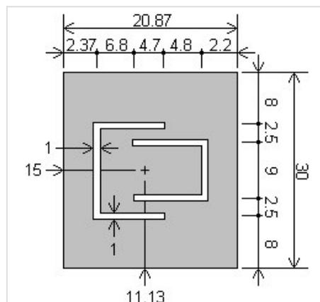
Fig. 4.6B.1 Parameters of the metallic patch of the designed dual-band antenna.
