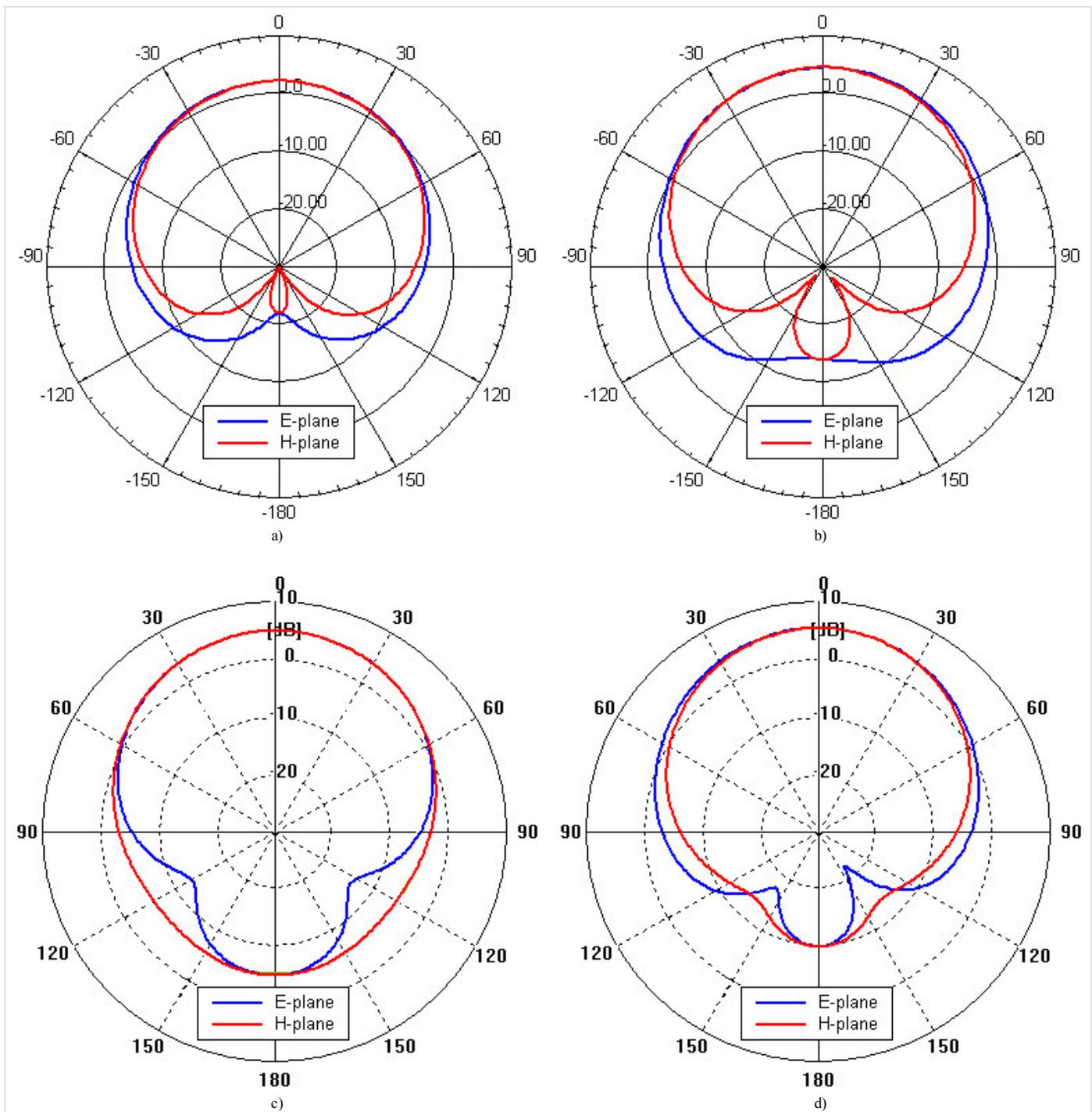
**Fig. 4.6B.5** Radiation pattern of the designed dual-band antenna: Ansoft HFSS,  $f_1 = 2,439$  GHz (a), Ansoft HFSS,  $f_2 = 3,600$  GHz (b), CST Microwave Studio,  $f_1 = 2,452$  GHz (c), CST Microwave Studio,  $f_2 = 3,588$  GHz (d).
