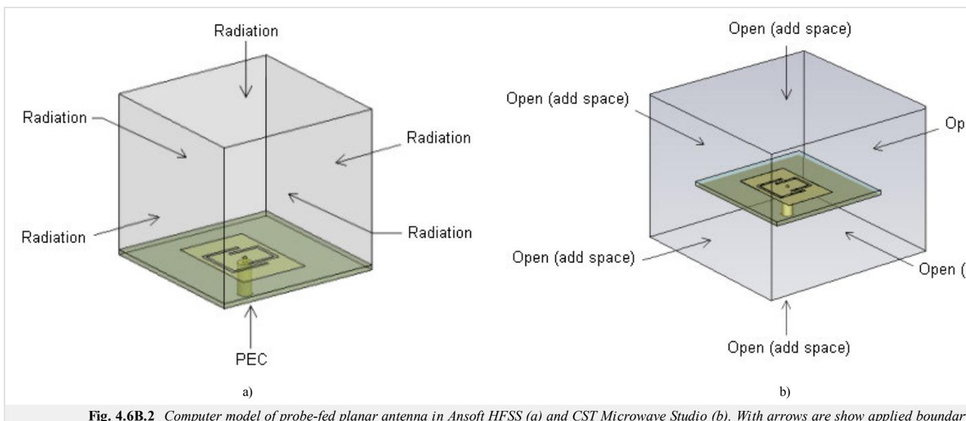
Fig. 4.6B.2 Computer model of probe-fed planar antenna in Ansoft HFSS (a) and CST Microwave Studio (b). With arrows are show applied boundary
