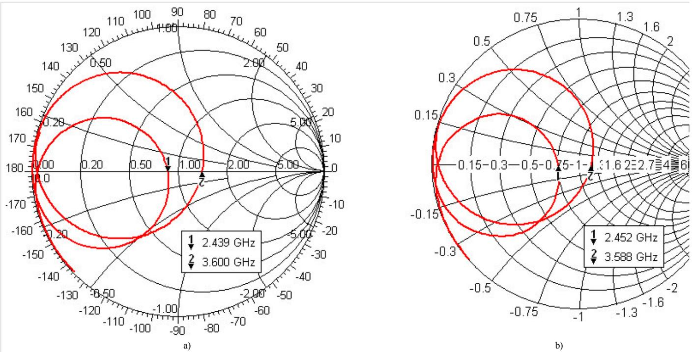
**Fig. 4.6B.3** Input impedance of the designed dual-band patch antenna in the Smith chart (from 2 GHz to 4 GHz): Ansoft HFSS (a), CST Microwave Studio (b)
