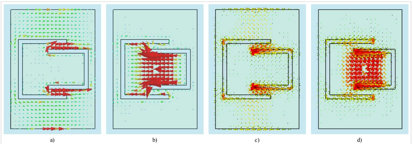
**Fig. 4.6B.4** Surface current density on the designed dual-band antenna: Ansoft HFSS,  $f_1 = 2.439$  GHz (a), Ansoft HFSS,  $f_2 = 3.600$  GHz (b), CST Microwave Studio,  $f_1 = 2.452$  GHz (c), CST Microwave Studio,  $f_2 = 3.588$  GHz (d). Red color – high density, blue color – low density.
