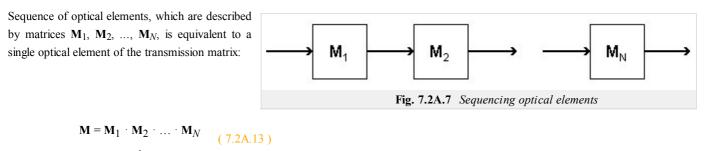
Note the order of the matrix multiplication. The matrix of the element, which is entered by the beam first, appears on the right, and therefore, it multiplies the column vector of the incident beam first.
