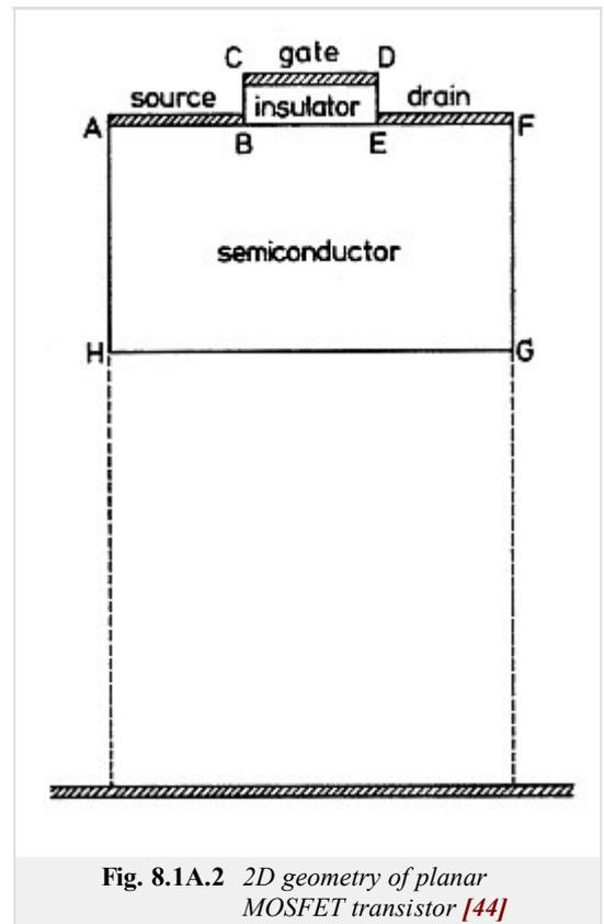
Fig. 8.1A.2 2D geometry of planar MOSFET transistor [44]
