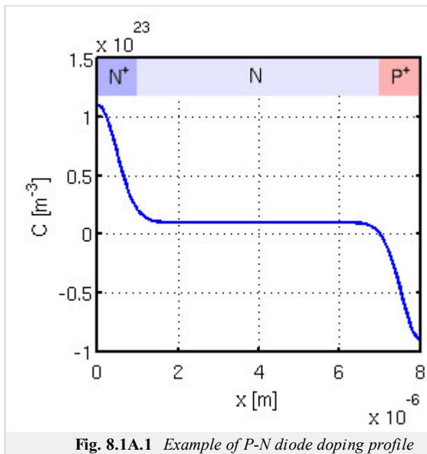
Fig. 8.1A.1 Example of P-N diode doping profile
