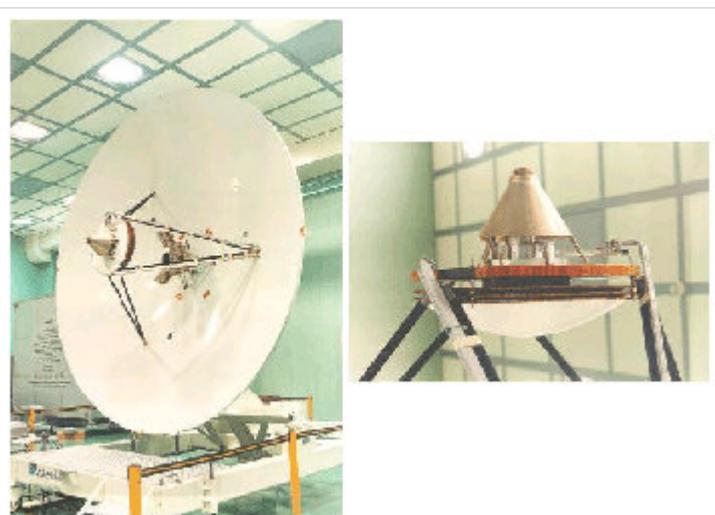
**Fig. 6.2** Antenna for the satellite Cassini 96 (left). A detailed view on hyperbolic sub-reflector of this antenna (right).
