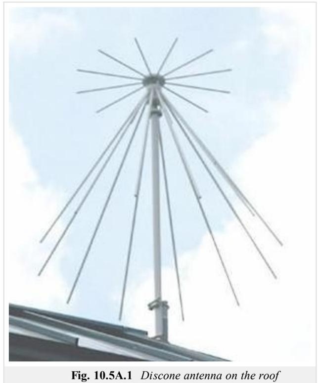
**Fig. 10.5A.1** *Discone antenna on the roof*
