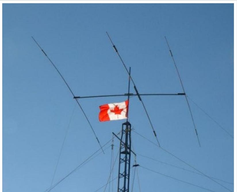
**Fig. 10.7A.1** *Practical implementation of Yagi antenna*
