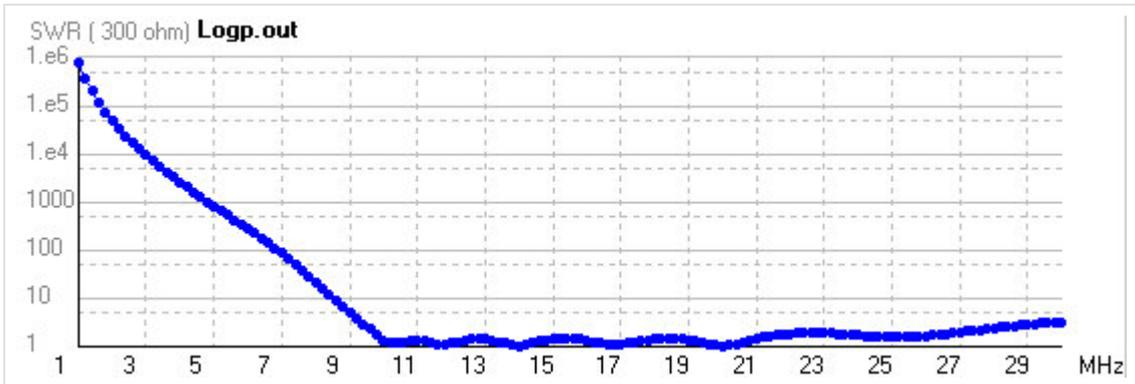
**Fig. 10.8A.3** Frequency response of standing wave ratio of LPA antenna (length  $d1 = 2.142$  m,  $d2 = 2.463$  m, spacing  $s1 = 1.143$  m,  $d3 = 2.833$  m,  $s2 = 2.803$  m,  $d4 = 3.255$  m,  $s3 = 4.713$  m,  $d5 = 3.741$  m,  $s4 = 6.903$  m,  $d6 = 4.299$  m,  $s5 = 9.833$  m,  $d7 = 4.941$  m,  $s6 = 12.313$  m,  $d8 = 5.682$  m,  $s7 = 15.633$  m,  $d9 = 6.531$  m,  $s8 = 19.463$  m)
